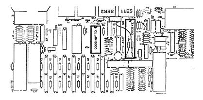
If your QL has a couple of little banded cylinders and bits of wire over the top of the ZX8302, this is mandatory modification "g". As this modification is very important in improving the reliability of the Microdrives, it has been incorporated onto the interface. The first thing you should do is to cut or break the wire and these "resistors" as close to the chip's legs as possible: wiggling the wires will usually do this quite well. Ensure that no bit of wire is left standing up.
