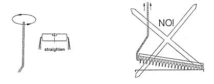
The legs of the two chips may be slightly splayed. Before trying to put the chips into the sockets on the interface, straighten the legs by pressing the side of the chip against the table top. If all the pins on the chips are straight, then, when the chips are rested on their sockets, the pins should be about half way into the sockets. If the chips are standing up slightly, re-straighten the pins.
