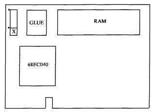
Smear a small amount of heat transfer compound onto the top of the 68040 and the bottom of the heatsink. Fit the heatsink onto the 68EC040 with the clips provided (it fits a treat). Connect the fan power supply with the
