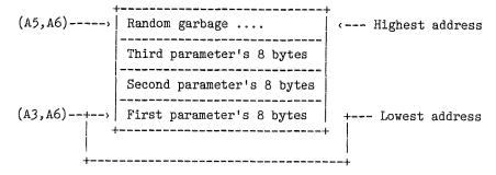
So (A3,A6) points to the first byte of the first parameter and is the lowest address, (A5,A6) points to the first byte past the last parameter and is the highest address.
